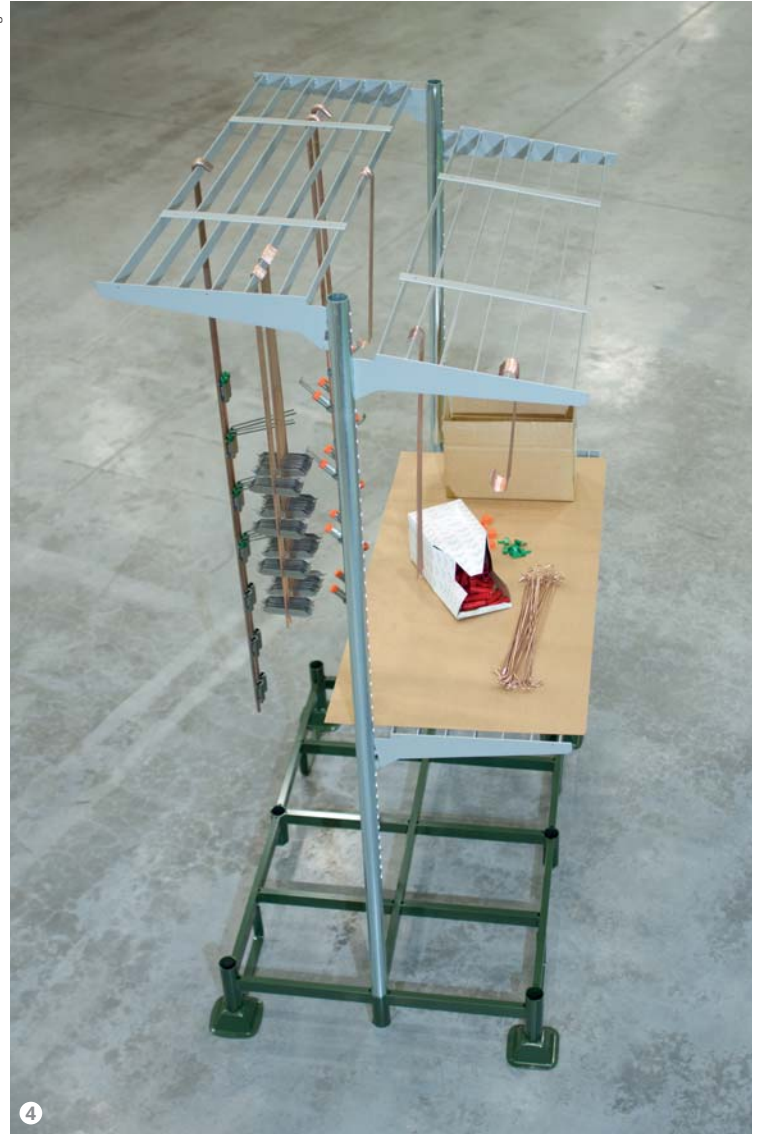
Figure 4: The shuttle can be used as a workbench for both material preparation and masking operations.
