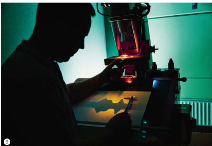
Figure 9: When testing a cap, its configuration, weight, and moulds' size consistency are checked.
