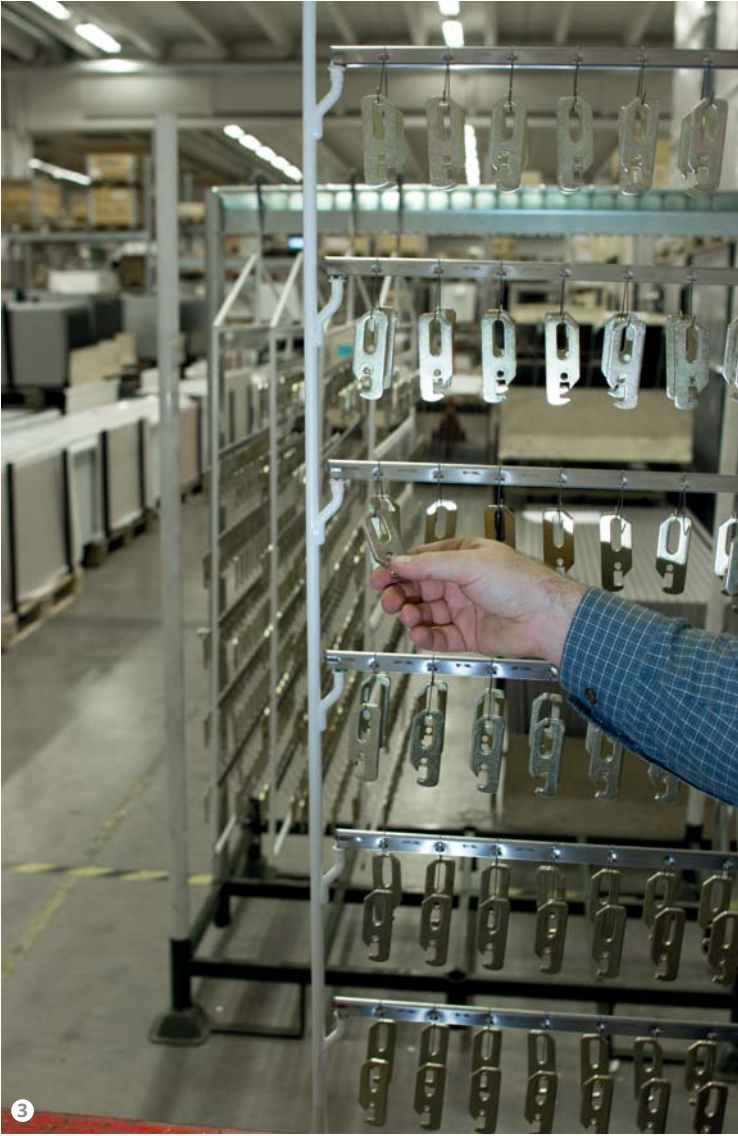
Figure 3: The frame also enables to unhang the workpieces, with due care and attention.
