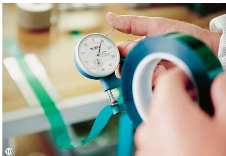
Figure 10: A control test on masking tape.
